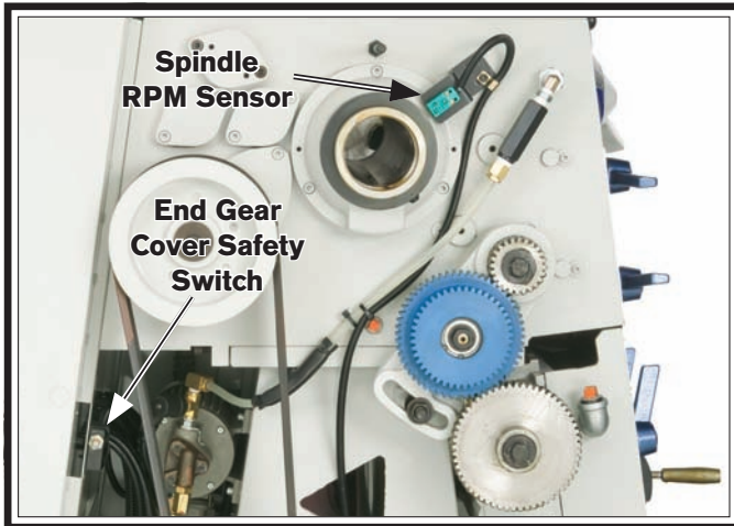
Figure 148. RPM sensor and end gear cover safety switch location.
